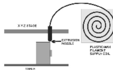
**Fig 4.** Schematic diagram showing fused deposition modelling.
