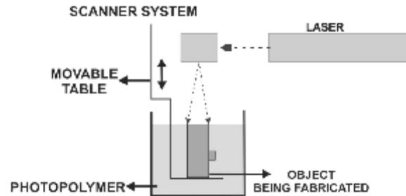
Fig 1. Schematic diagram showing stereolithography procedure.
