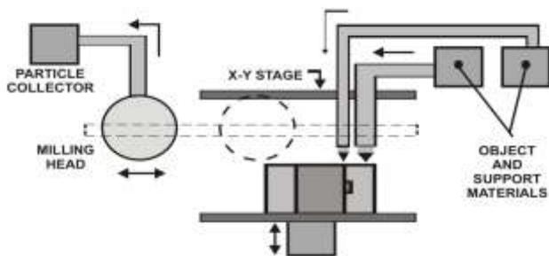
**Fig 5.** Schematic diagram showing Inkjet (Thermal phase change) procedure.
